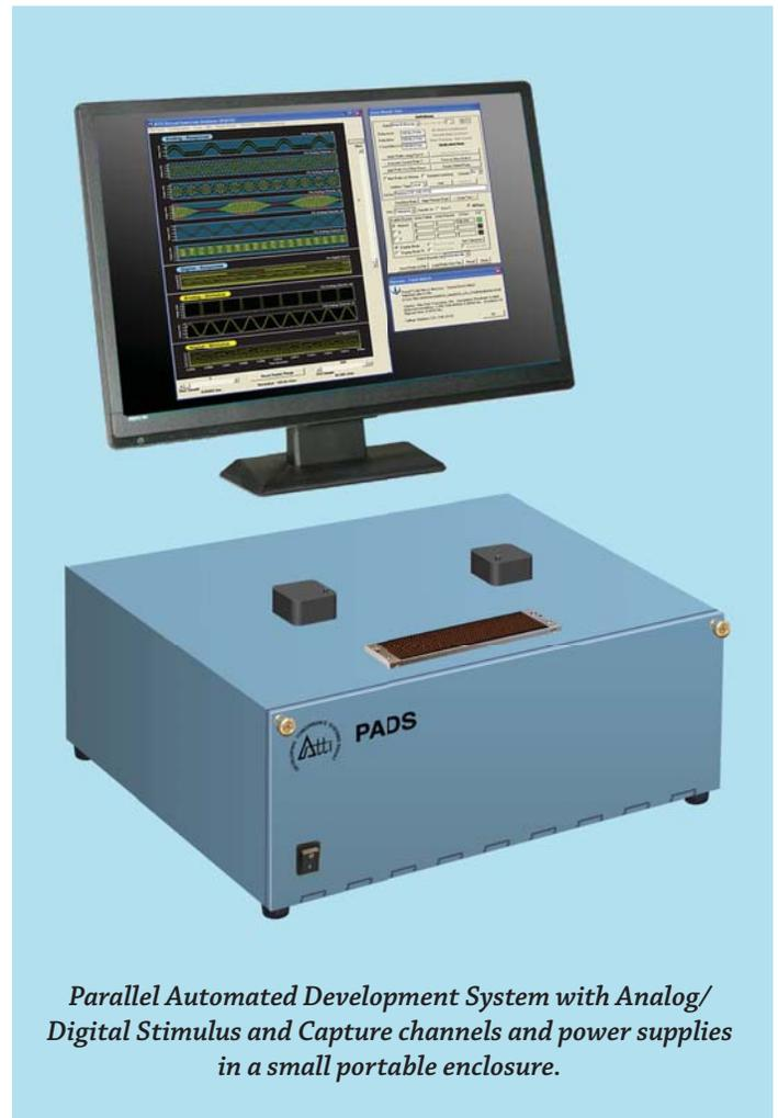
*Parallel Automated Development System with Analog/ Digital Stimulus and Capture channels and power supplies in a small portable enclosure.*
